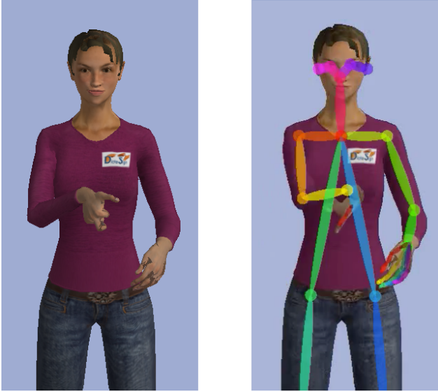
Figure 5: Example of body keypoints (on the right) extracted from a single animation frame (on the left)
